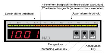
Fig. 4 Description of the NA3 frontal plate.
